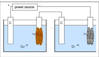
Example 6 A charge of 0.250 Faraday was passed through an electrolytic cell with 0.100M solution of  $CuSO_4$ , as shown on the right.
